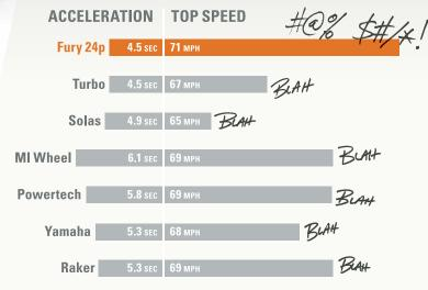
All runs measured using a Triton TR-21X with 225 OptiMax ProXS under same conditions. Acceleration time is from 0-20 MPH.
